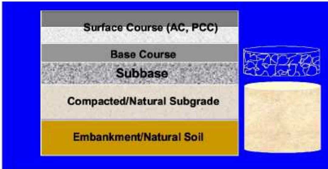
Figure 1-1. Basic components of a typical pavement system.
